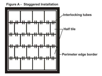
The correct installation of Dinoflex Rubber Tiles is a staggered pattern to ensure proper alignment, a tighter fit, and reduction of vandalism.
